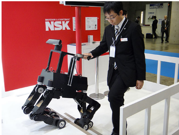
(a) NSK robotic guide dog for the visual impaired 1 .
