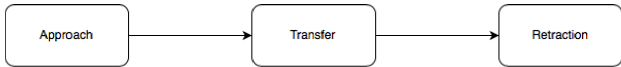
Figure 2.8: Object handover schematic phases.
